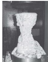
Fig. 2. Fractured test specimen at failure.
